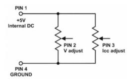
Two variable resistors must be set up at the same time in order for the remote control to be functional.
