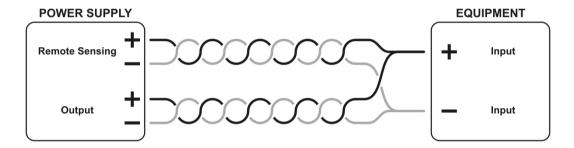
The remote sensing wire should be AT LEAST 22AWG wire size.
