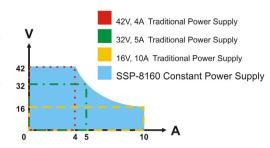
A conventional power supply only has a set of maximum voltage and a set of maximum current such that all the operating V & A must fall inside these limits.
