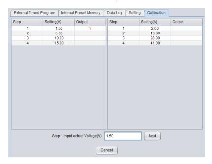
There are total 8 steps for calibration. 4 steps for Voltage and 4 steps for Current. You only need to follow step by step to finish calibration.
