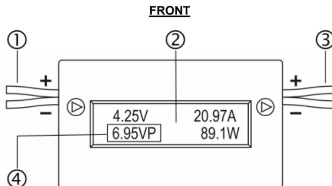
① Bidirectional terminal for simultaneous connections to load & source.
