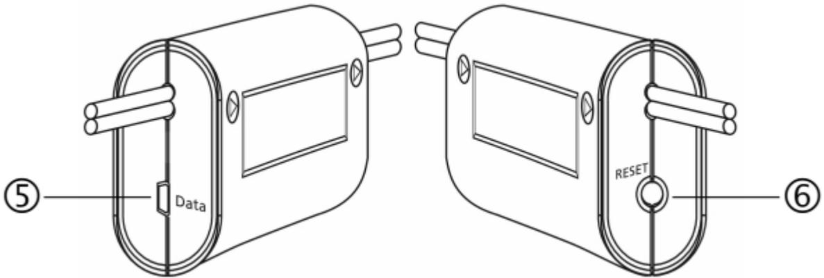
⑤ Micro USB socket : Either for connection to PC for data retrieval & real time monitoring.
