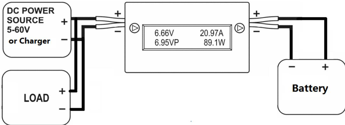
**Bi-directional application with external DC for 0-60V meter range**
